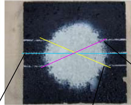
Evaluate the area where the thickness of the adhered neutron absorber meets the prescribed coating thickness (tentatively set to 1 mm)
