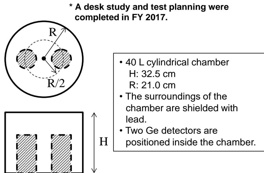
Figure 2 - (Proposed) Chamber Profile of the Enhanced System
