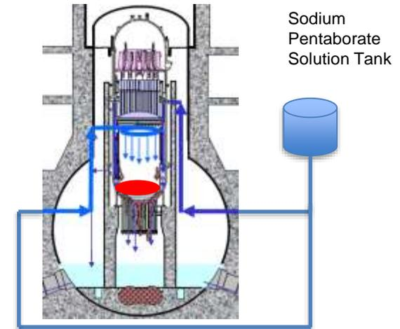
Figure 3 - Criticality Termination Model
