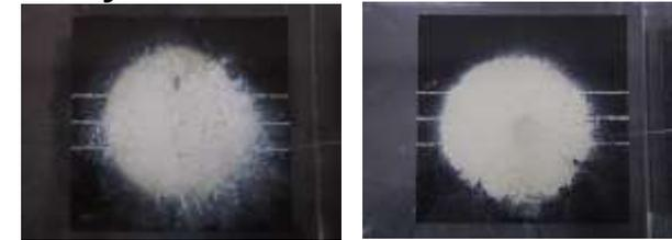
Image of Neutron Absorber Adhered to Plate Lava (Temperature: 20 °C)
