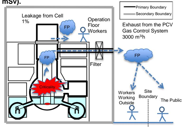
Figure 4 - Exposure Model Caused by Criticality
