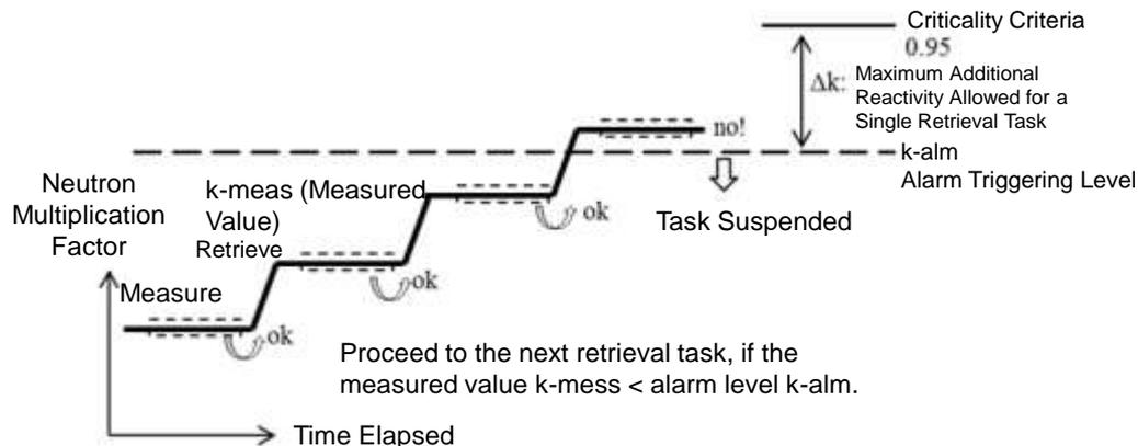
Figure 1 - Image of Criticality Prevention Through Critical Approach Monitoring
