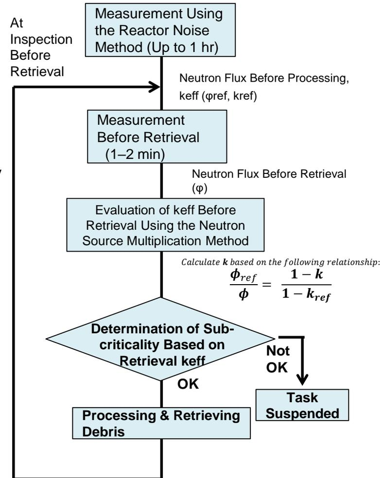
Figure 2 - (Proposed) Critical Approach Monitoring Flow
