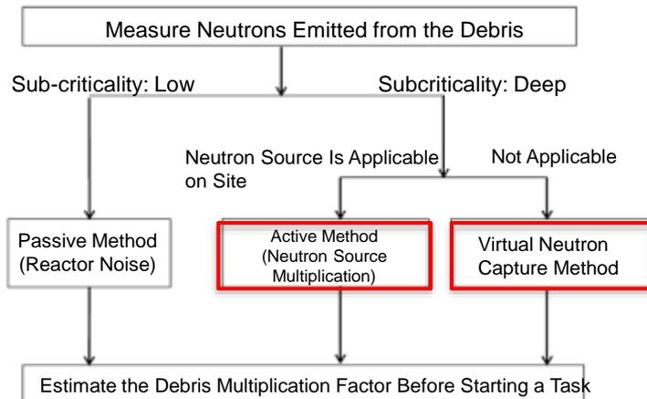
Figure 2 - Flow Chart of Critical Approach Monitoring Technologies
