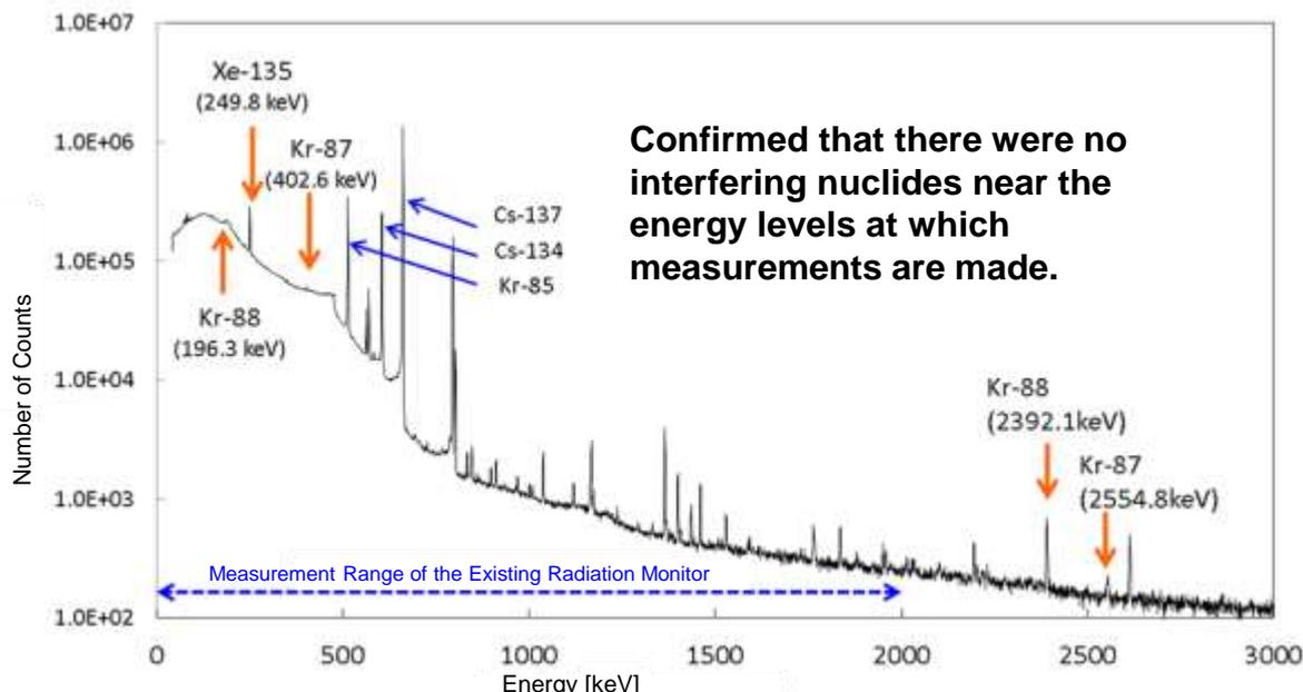
Figure - Unit 1 Gamma Ray Spectrum Measurement Results (Total)
