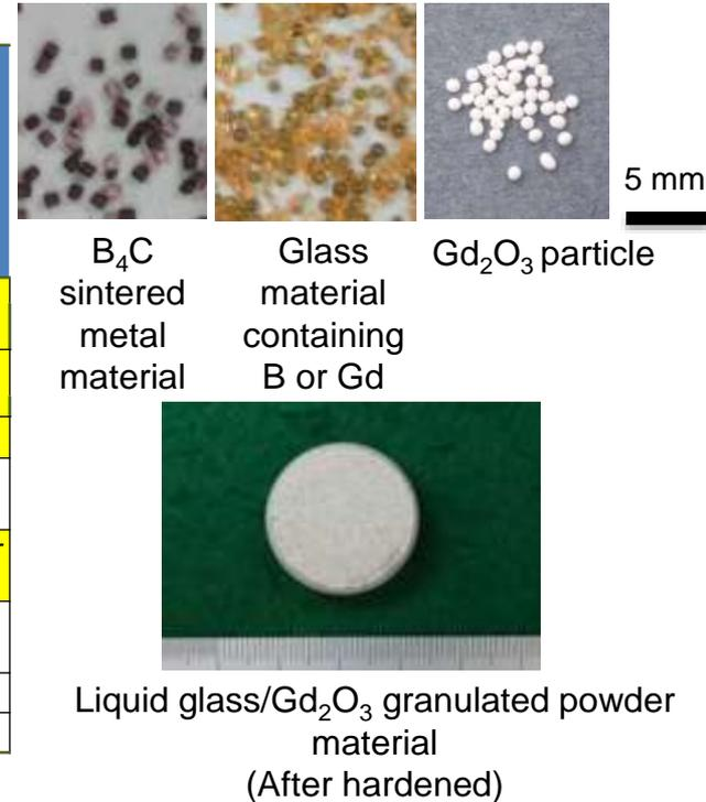
Candidate materials were selected as one of the accomplishments in FY 2017, based on the results of confirmation of neutronics, a long-term irradiation test, and a workability test (shaded in yellow).
