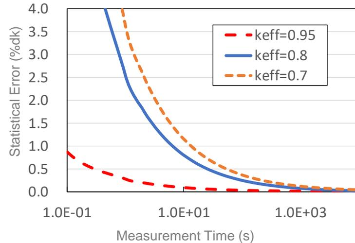
Figure 3 - Correlation between Measurement Time and Statistical Error
