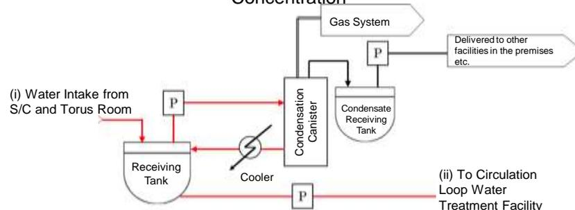
Figure 2 - Boron Condensation System with Condensed Canister
