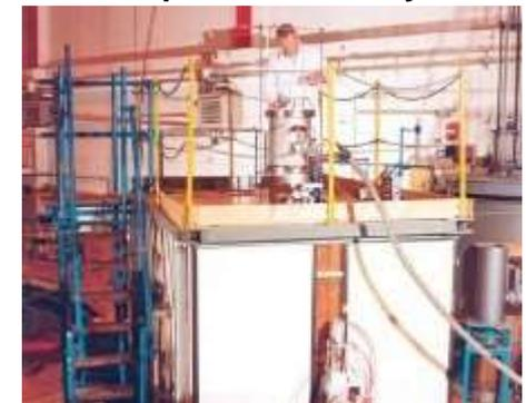
Figure 3 - Thermal Neutron Pile
