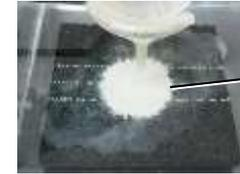
Neutron absorber flowing down while expanding in the water
